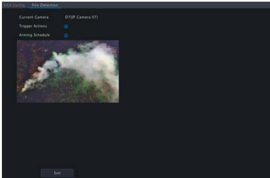
4. Set the alarm-triggered actions and arming schedule. See [Alarm-triggered Actions](#) and [Arming Schedule](#) for details.
