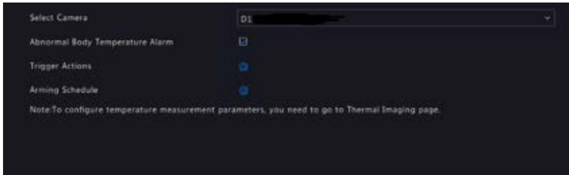
2. Select the infrared light channel, and enable **Abnormal Body Temperature Alarm**.
