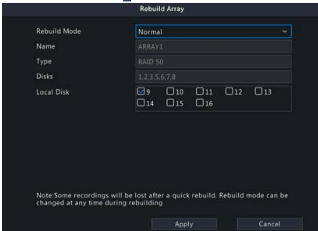
3. Select the rebuild mode and local disk. The **Quick** rebuild mode takes less time than the **Normal** rebuild mode, but may result in data loss. Please select with caution.
