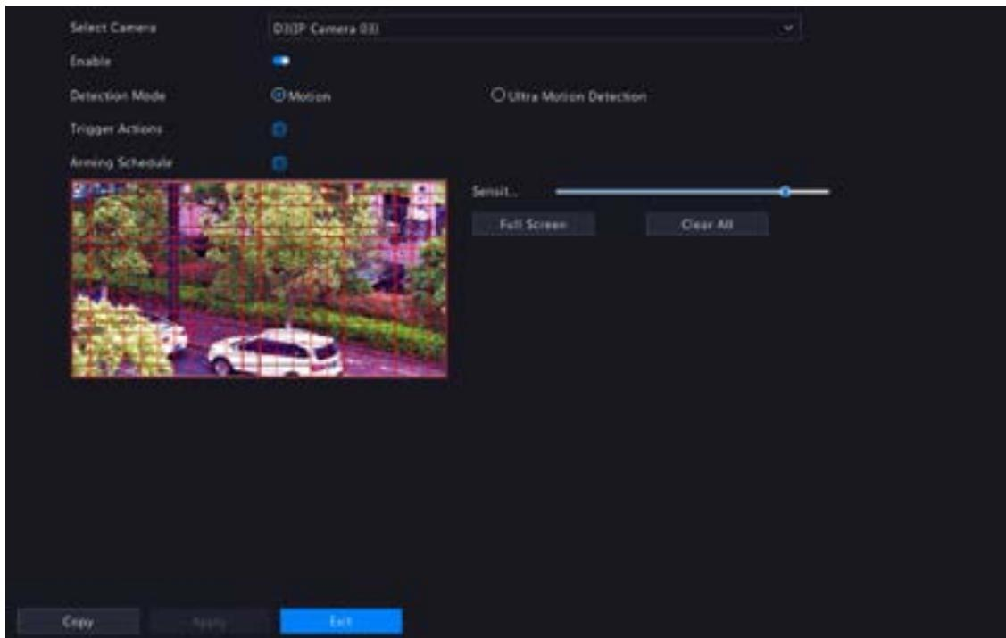
2. Set the detection area. The default is the full screen. You can adjust grid detection areas as needed.
