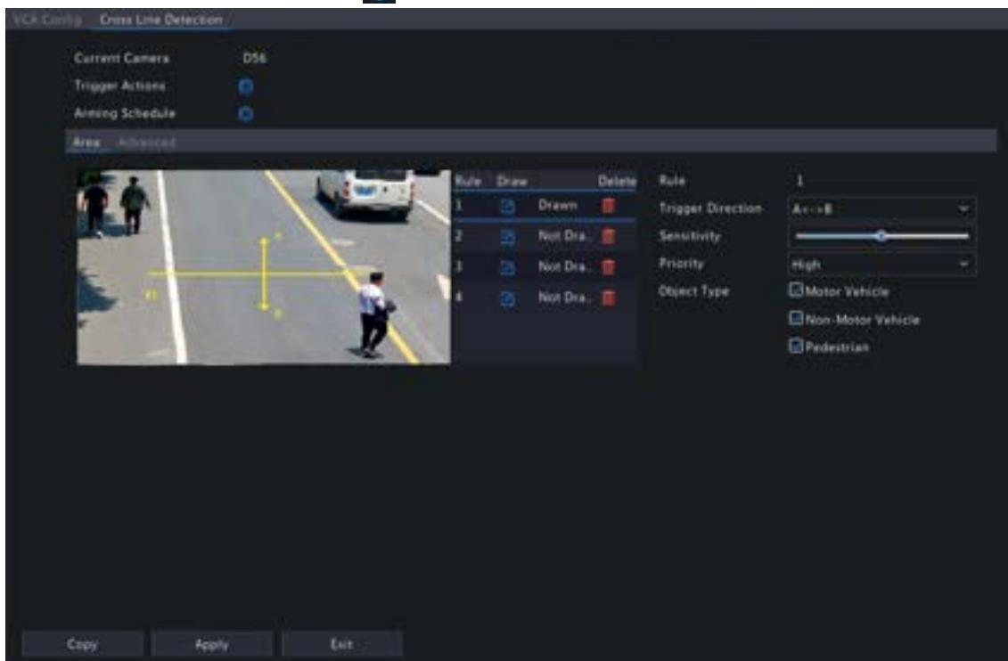
4. Set detection rules. The 4 detection rules shall be set separately. The following takes Rule 1 as an example.
