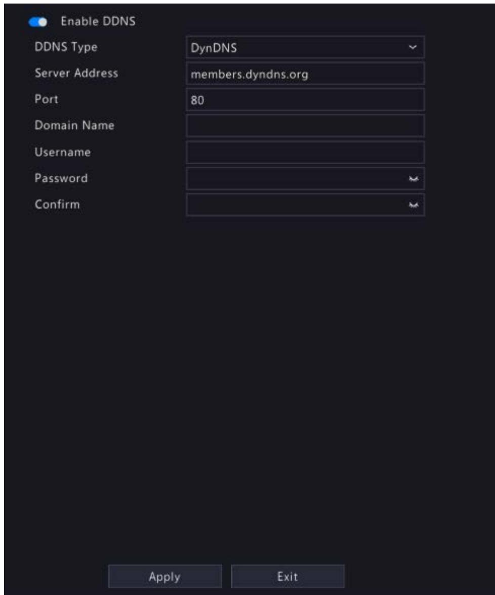
2. Enable DDNS, choose a DDNS type, and configure the parameters.
