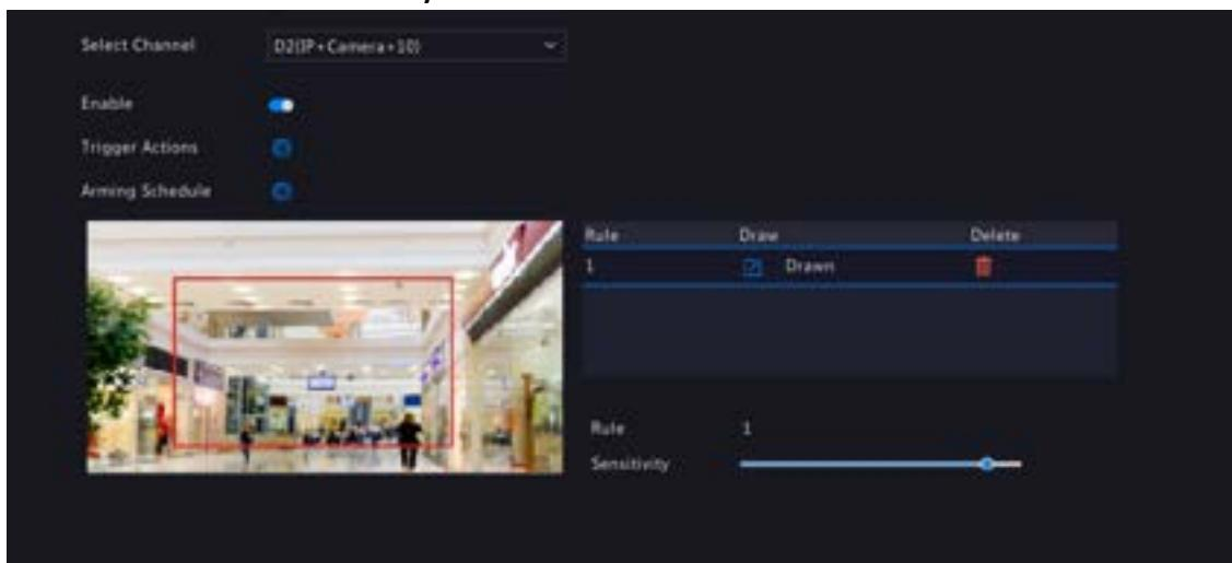
2. Select the desired channel, and enable human body detection.
