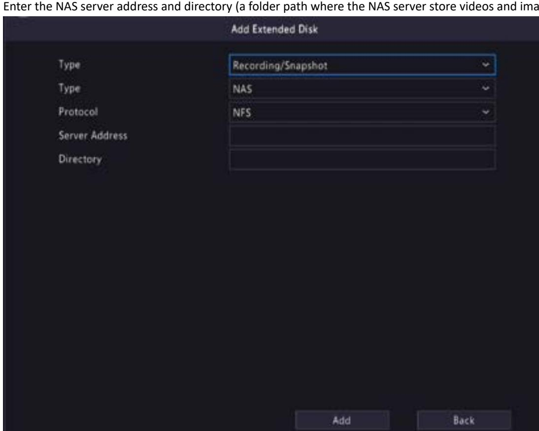
The screenshot shows the 'Add Extended Disk' configuration page. The 'Type' dropdown is set to 'Recording/Snapshot'. The 'Protocol' dropdown shows 'NAS' as the selected option. The 'Server Address' and 'Directory' fields are empty. At the bottom are 'Add' and 'Back' buttons.
