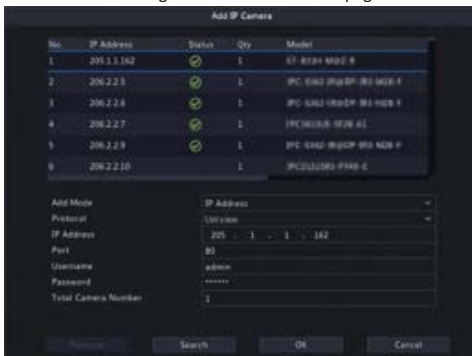
(3) Set the add mode to **IP Address**, select a protocol, enter the IP address, port, username, and password. There are 2 channels in total, including a visible light channel and an infrared light channel.
