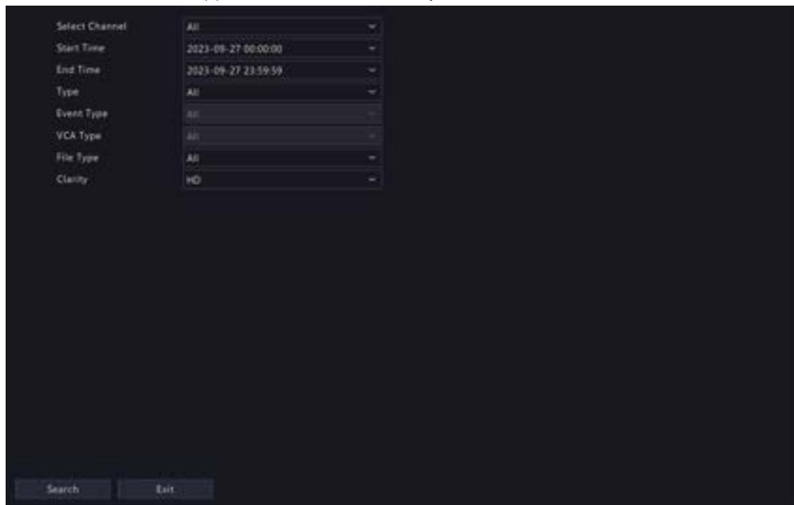
3. Set search conditions, including the start time, end time, recording type, event type, VCA type, file type, and clarity (HD or SD).
