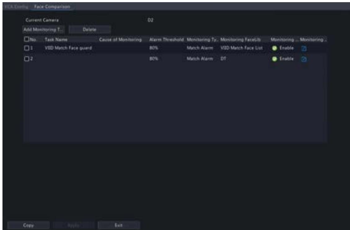
4. Configure monitoring tasks. A monitoring task of "DefaultList 80% Match Alarm" is enabled by default. You can click  to modify it, or click **Add Monitoring Task** to add more.
